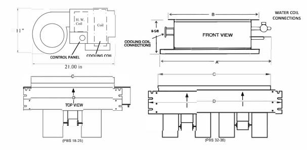
Copper stub out diameter: DX - Suction: 3/4", Liquid: 3/8"; Hydronic – Water In/Out: 7/8"
