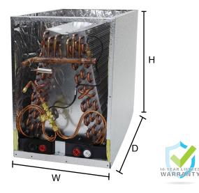
Unit shown with service panels removed. Representative image only. Some models may vary in appearance. Duct opening dimensions can be ascertained by subtracting 1-1/2" for top opening width/depth, 3/4 for bottom opening. Due to continous product improvement, specifications are subject to change without notice.
