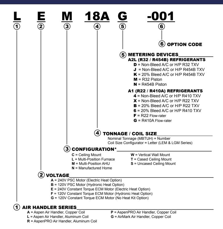
\*A2L wall and multi-position air handlers are supplied with factory installed refrigerant detection systems; ceiling mount air handlers are supplied with a field installed refrigerant detection system kit.
